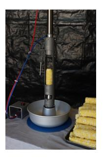
The Funnel only advances as long as the button on the Control Box is held depressed. As soon as the operator releases the button, the cylinder will retract at a rate metered by the flow control valves, no matter where it is in its stroke.
